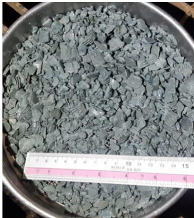
Figure 2. Cuttings from shale shaker clearly showing preserved condition, illustrating the superior inhibition achieved from utilizing the customized HPWBM system
