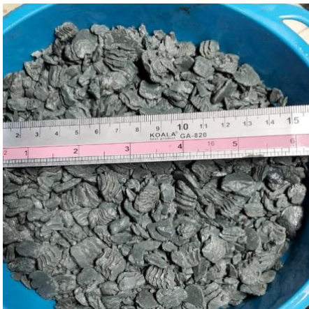
Figure 2. Cuttings from shale shaker clearly showing preserved condition, illustrating the superior inhibition achieved from utilizing the customized HPWBM system
